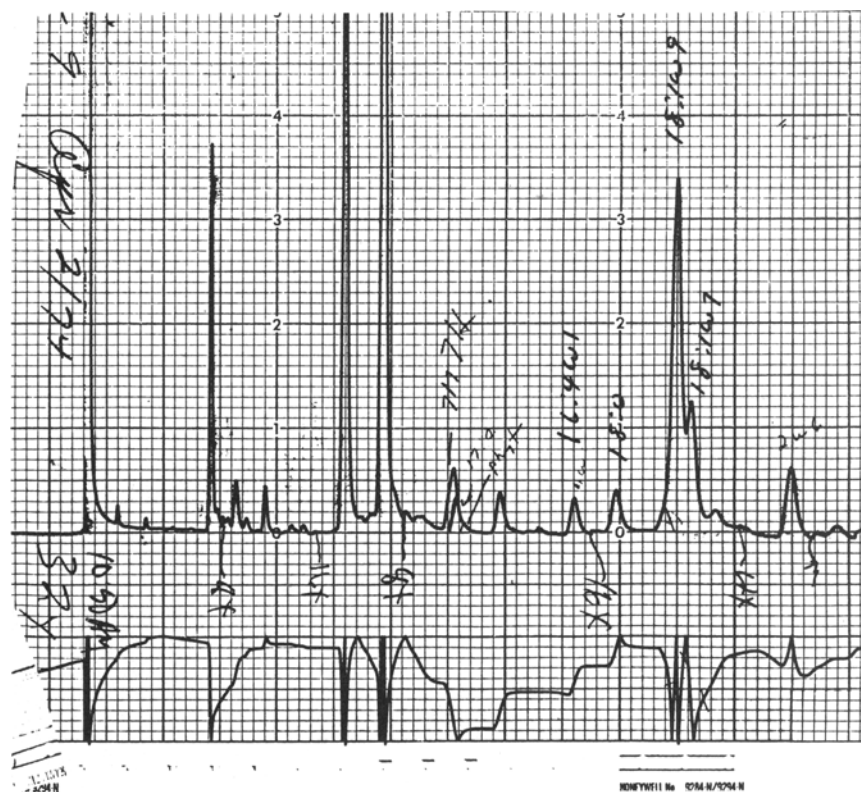
FIG. 2. The original early part of a chromatogram of the analysis in 1974 of the methyl esters of fatty acids from a fish (capelin) oil on a Perkin-Elmer stainless steel column, 0.01 inch i.d. \times 150 ft operated at 180°C with He carrier gas at 60 psig. The first three large peaks are 14:0, 16:0 and 16:1n-7. Note shoulder for 18:1n-11 before 18:1n-9 and small 18:1n-5 peak after 18:1n-7. Time to 18:2n-6 (linoleic acid) peak was 17 minutes.
